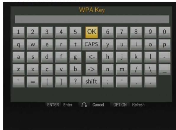
Encryption keys can be inputted via the virtual keyboard. Press the navigational buttons to select, **ENTER** to input, **CAPS** to switch between uppercase and lowercase, **<-** to delete a character, **->** to insert a space, **shift** to make more symbols available, and **OK** to confirm.
