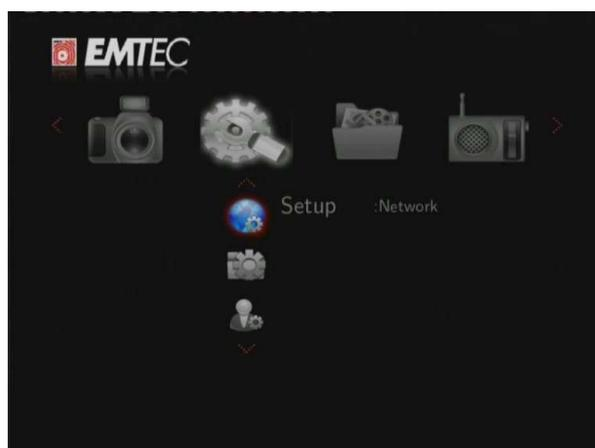
There are five Setup options, including **Audio**, **Video**, **Network**, **System**, and **MISC**. Use the **UP/DOWN** navigational buttons to select a menu. Press **ENTER** to confirm. Press **RETURN** to cancel and display the previous menu screen.
